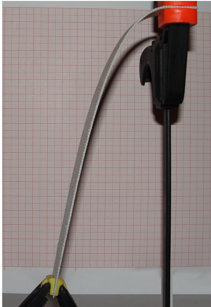
(a) Displacement after clamping the soft side and attaching a weight to the hard side
