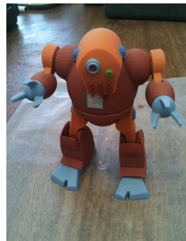
(d) Finished part after excess powder is removed
