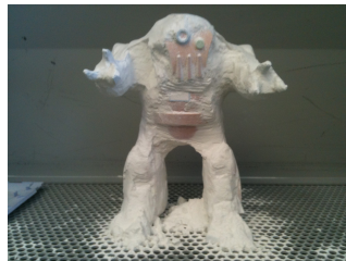
(c) Finished part with excess powder
