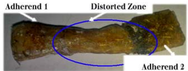
Figure 4. Distorted joint due to excessive exposure time
